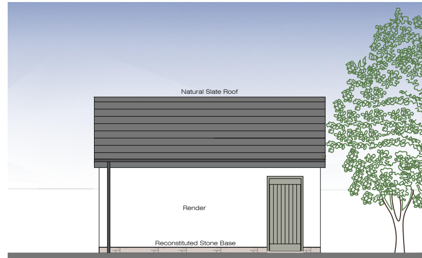
Side Elevation Single Garage
